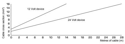
Connect your cooling device as directly as possible to the battery terminal or to an outlet with a fuse of at least 15 A (12 V) or 7.5 A (24 V).
